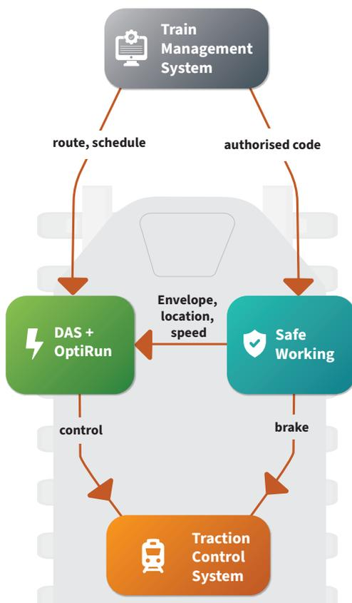
The **Traffic Management System (TMS)** is responsible for managing all the trains on a network. Each train (orange box) has a Safe working unit, a Driving Advice System (DAS) and a Traction Control System.
